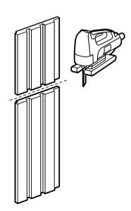
Panels can be mounted vertically, horizontally, and diagonally. If you want to trim them, use a handsaw, jigsaw, or table saw.
