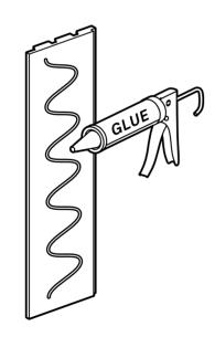
Apply adhesive on the back of the panel in the shape of the letter "S", then attach the panel to the wall.
