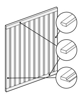
To finish the wall, use the system trims, which, like panels, are mounted with adhesive. For each of the panel types, you can choose the right and left trims, while the universal trim will allow you to finish the top and bottom of the wall.
