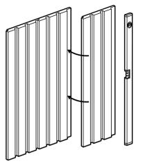
Always lay the panels starting from the left and then moving right and starting from the bottom, moving up.
