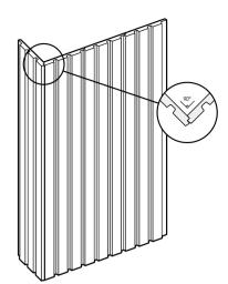
Remember to connect the panels carefully in the outer corner. All you have to do is slot them in one another at 90 degrees.
